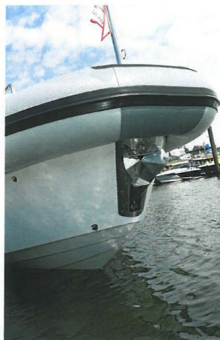
Vertical stems seem all the rage these days – especially when they house a hidden anchor.
